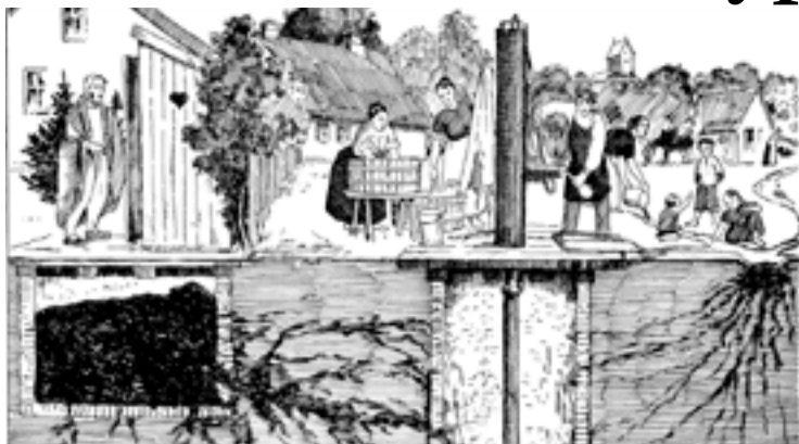
An illustration showing various ways that a water well may become infected by typhoid fever bacteria. Photo: SUPPLIED
